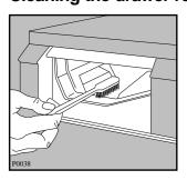
Having removed the drawer, use a small brush to clean the recess, ensuring that all washing powder residue is removed from the upper and lower part of the recess.
